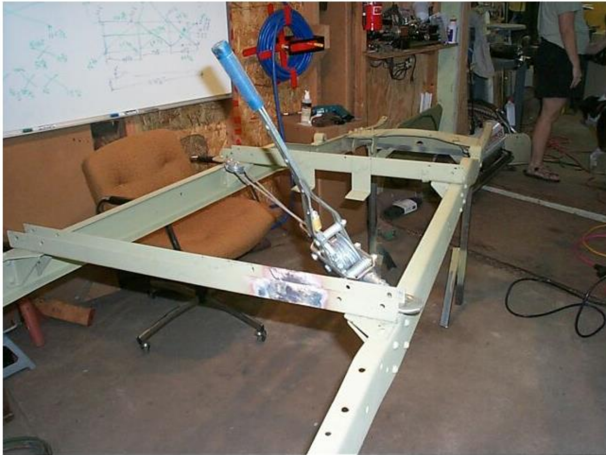
repair of bent frame Image 16 of 18
