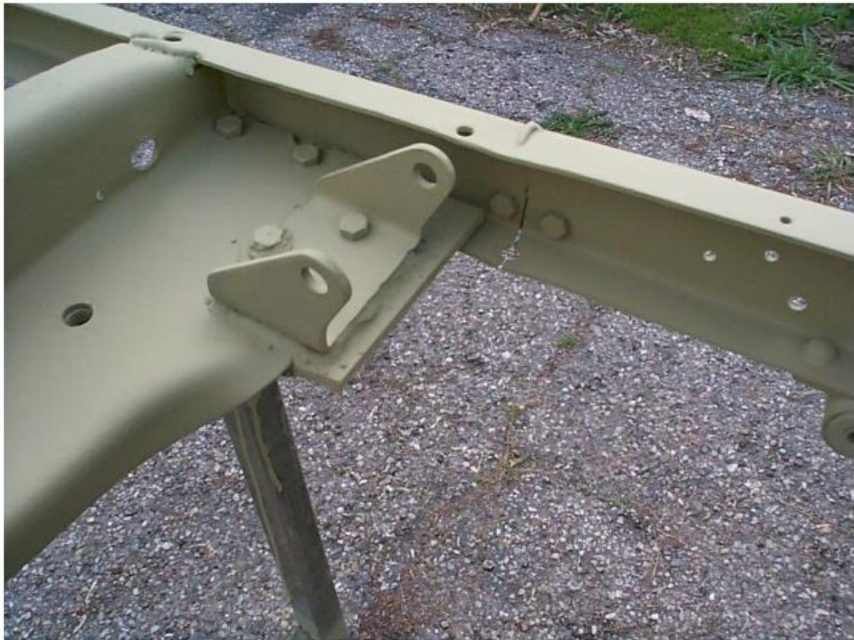
the steering gear bracket and the crack in the frame
