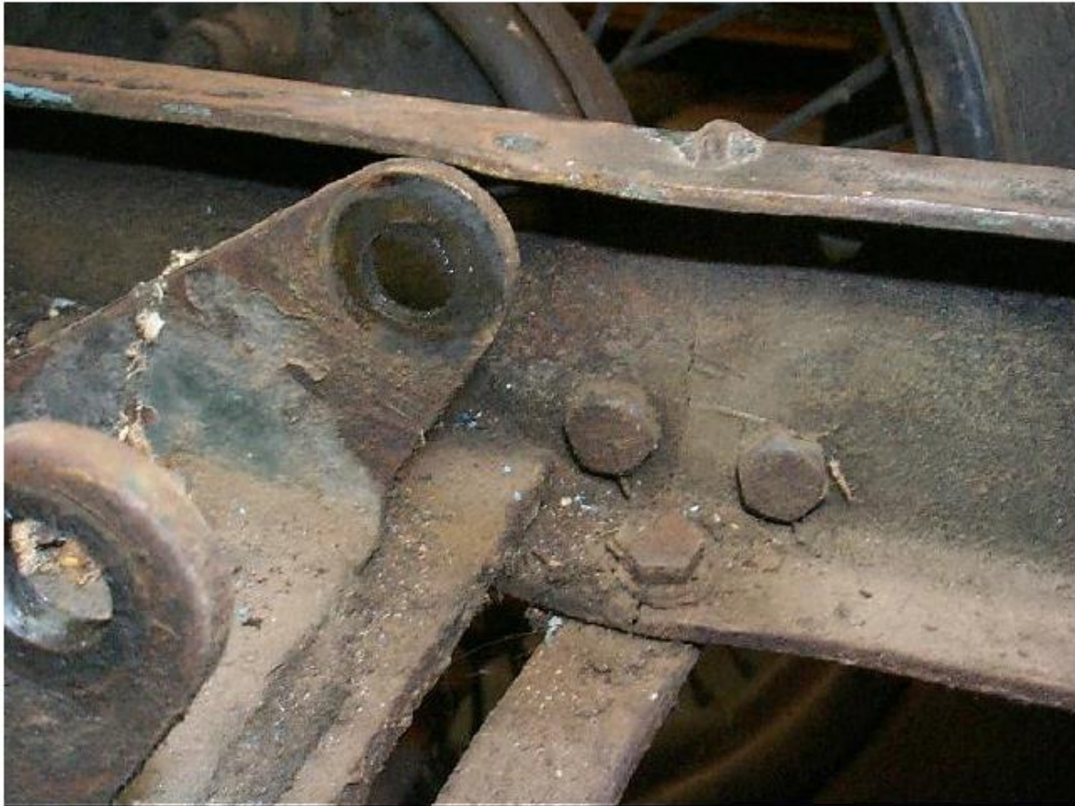
the first view of the crack in the frame
