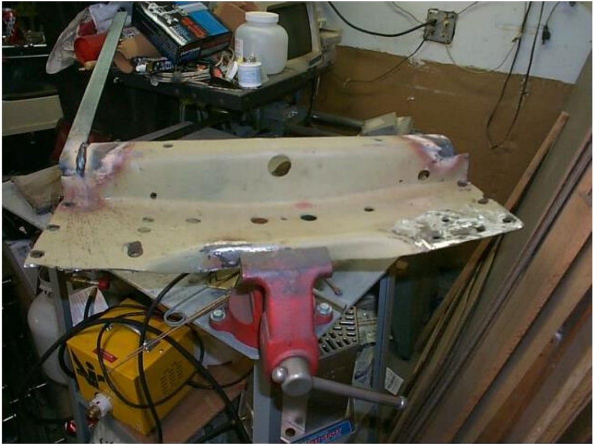
welding/repair of front crossmember Image 13 of 18
